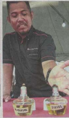
Uni10 Energy operations supervisor Yahirwan Yahya shows the difference between biodiesel made from recycled cooking oil (left) and fossil diesel (right) in a burning demo. The fossil diesel gives off more black smoke.
